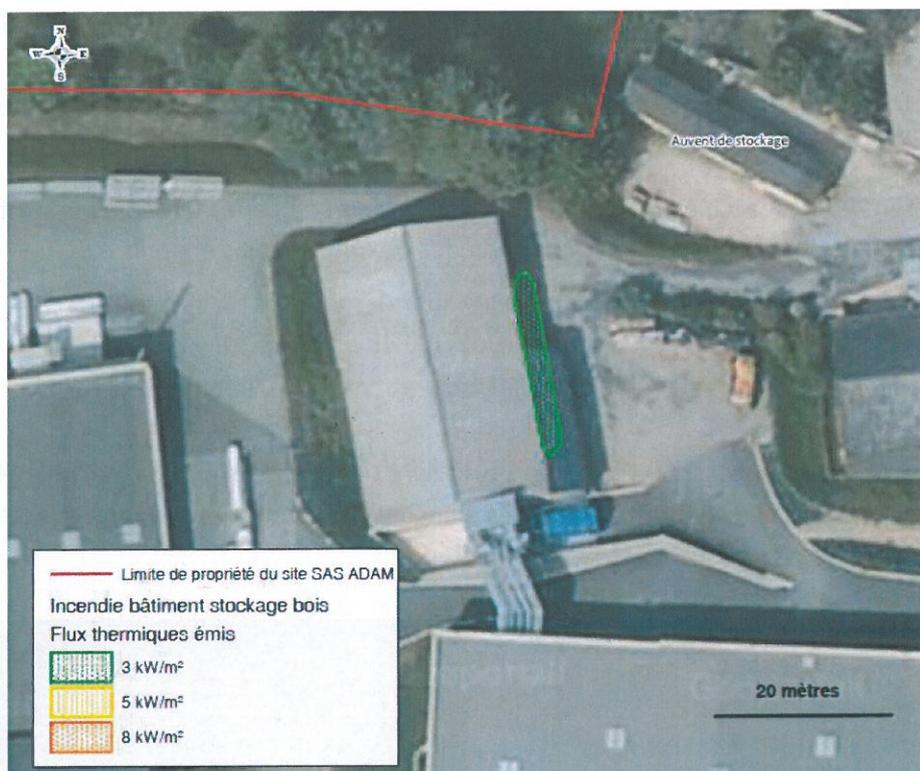
FIGURE 8 : SC\_18 - CARTOGRAPHIE DES ZONES D'EFFETS DES FLUX THERMIQUES
