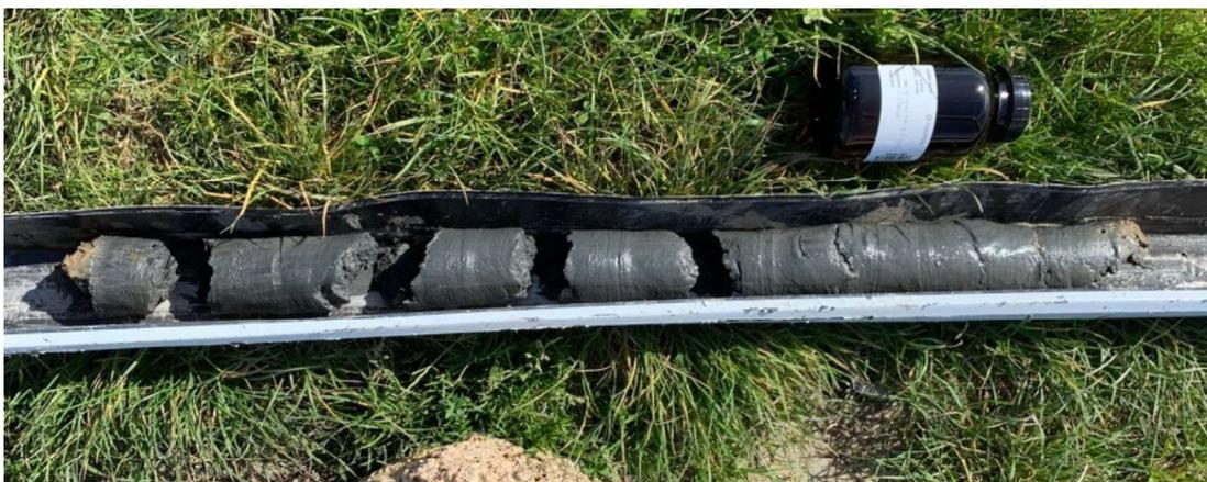
A photograph showing a sediment core sample labeled E1. The core is dark grey and appears to be composed of several segments, possibly held together by tape or a core catcher. It is placed on a metal tray or container. A small black bottle with a white label is visible in the background, likely used for sample collection or storage. The background is green grass.  |
