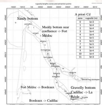
Fig. 2: Initial partition of bottom friction coefficient
