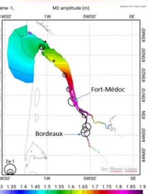
Fig.3: M2 amplitude (Complex, (m)) over Gironde color scale; M2 amplitude. Difference model - tide gauge (circle size in cm) (MarEst Project, Shom, Legos)
